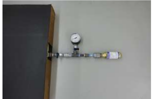
Figure 11: 25 Gram N 2 Gas Cylinder for VRIIB Inflation
