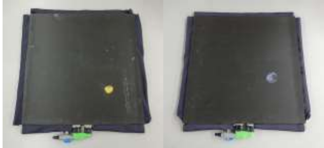
Figure 10: Chalk Marks on VRIIB Surface After Helmet Shell Impact – Blast Test #3
